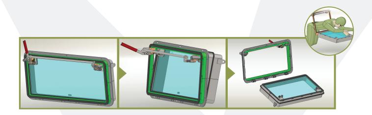
OSG's EEWS solution operates efficiently regardless of vehicle position, offering egress route when doors are blocked.
